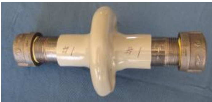
Fig. 2 A New Coated Flanged Sample, steel tube OD= 1.325", both ends capped with some bare metals exposed
