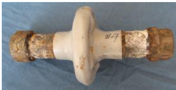
Fig.3E Flange #4 – After 3,000 Hr Salt Fog
