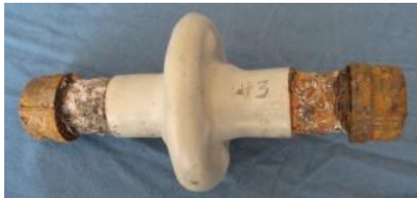
Fig.3C Flange #3 – After 3,000 Hr Salt Fog
