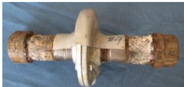
Fig.3F Flange #4-After 3,000 hr Sal Fog with a Cutout
