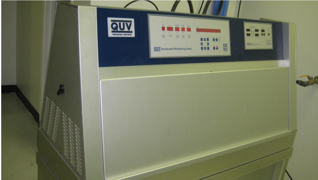
Fig 1 QUV Chamber for the ASTM G53 UV/Condensation Exposure
