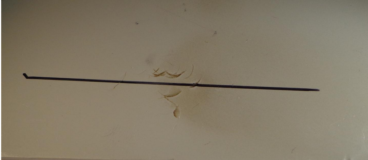
Fig 4 Oxifree TM198 Coating after ASTM D968 Sand Abrasion Test
